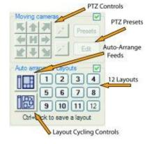
The second section controls the appearance of cameras on-screen and provides for 12 individually customisable layouts. Each layout can be setup manually and saved, enabling **rapid switching between layouts**.
